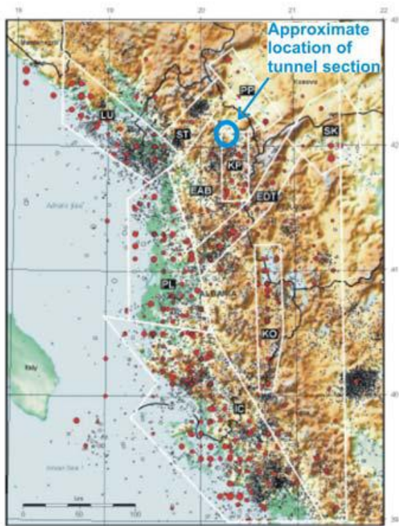
Historical and instrumental record of seismicity in Albania (from Aliaj et al., 2004). Red: historical catalogue, grey: recent catalogue since 1964. Magnitude range from 2.0 to 7.0
