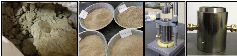
Figure 1. Soil pulverization process and specially manufactured split mold for sample preparation
