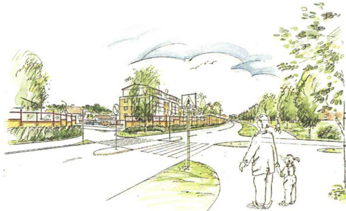
Pedestrian crossing located close to a three-leg intersection
