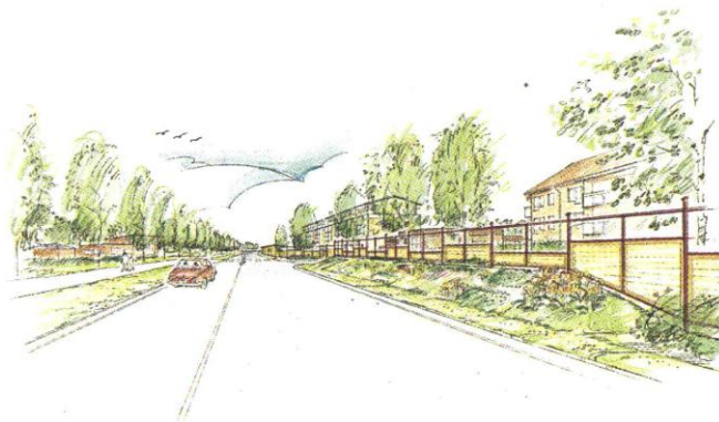
Cross-section showing separated pedestrian lane (left) and fence between the road and a residential area (right).
