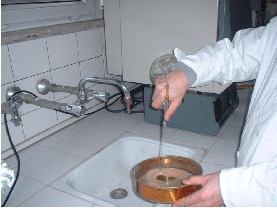
KİMYA LABORATUVARI, AGREGADA SİLİS TAYİNİ DENEYİ
