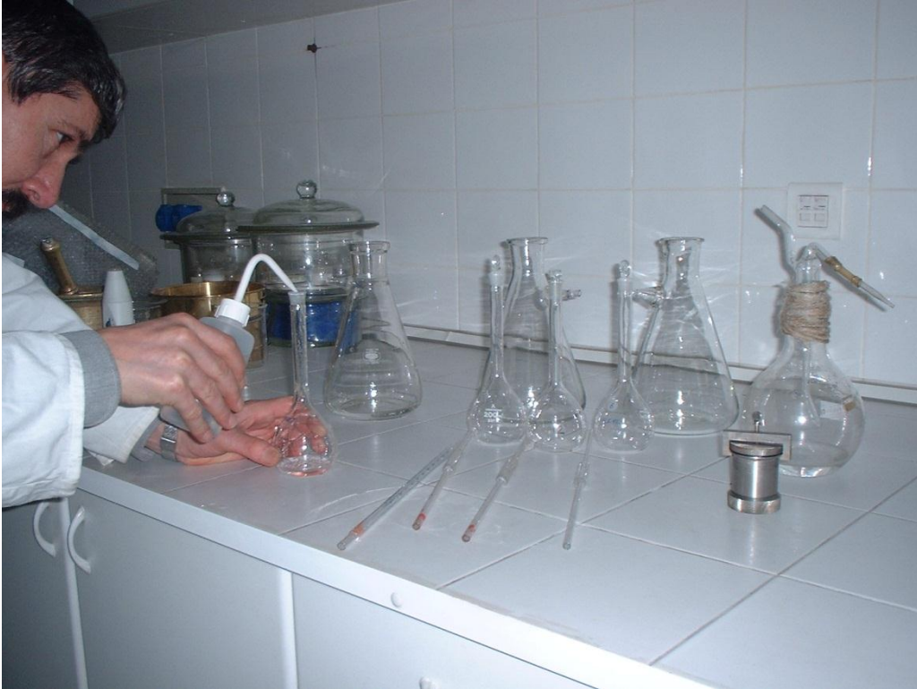
KİMYA LABORATUVARI AGREGADA ALKALİ TAYİNİ DENEYİ
